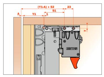
Height adjustments +2.5 mm Depth adjustments +/- 3 mm Side adjustments +/- 1.5 mm
