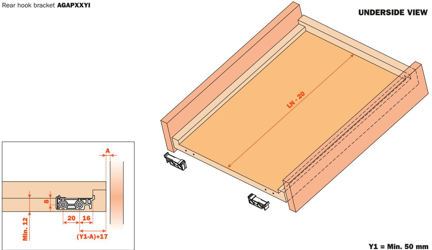
Assembly on the pull-out shelf with a 16 mm minimum thickness
